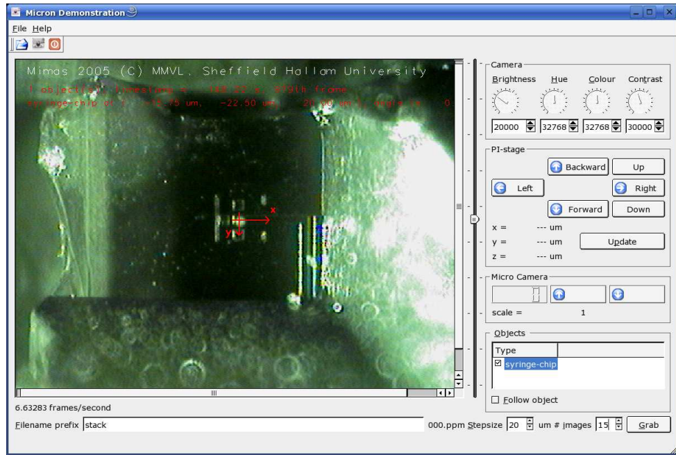
Figure 1.5: The graphical user interface of the recognition and tracking software. The x - y axis frame indicates the position of the recognised and tracked syringe chip. The image has been taken with a optical microscope and its quality is better than the images obtained with the MiCRoN camera.
