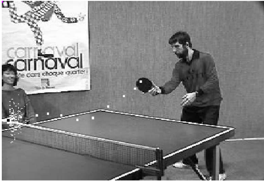
Figure C.1: Tracking of a ping-pong ball. Top left corner, the ball template image. The large white dots represent the previous tracked positions of the ball. The large black dot, the current position of the ball and the small white dots, the particles' positions.
