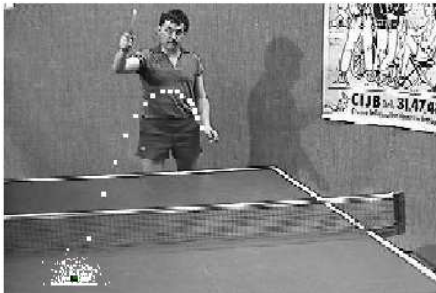
Figure C.1: Tracking of a ping-pong ball. Top left corner, the ball template image. The large white dots represent the previous tracked positions of the ball. The large black dot, the current position of the ball and the small white dots, the particles' positions.
