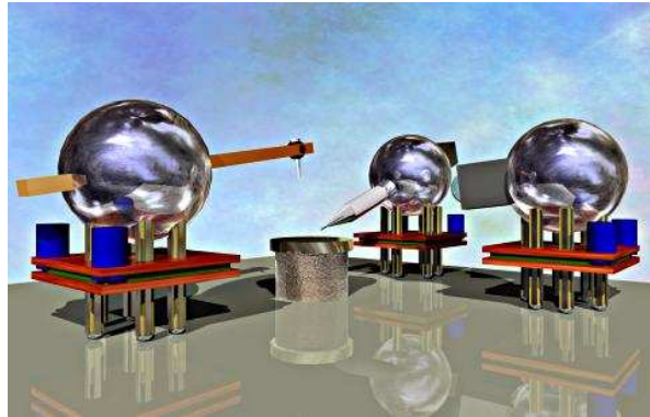
Figure 1.1: An artist impression of the MiCRoN project made for the project proposal: mini robots, 1 cm across, working cooperatively in an assembly task
