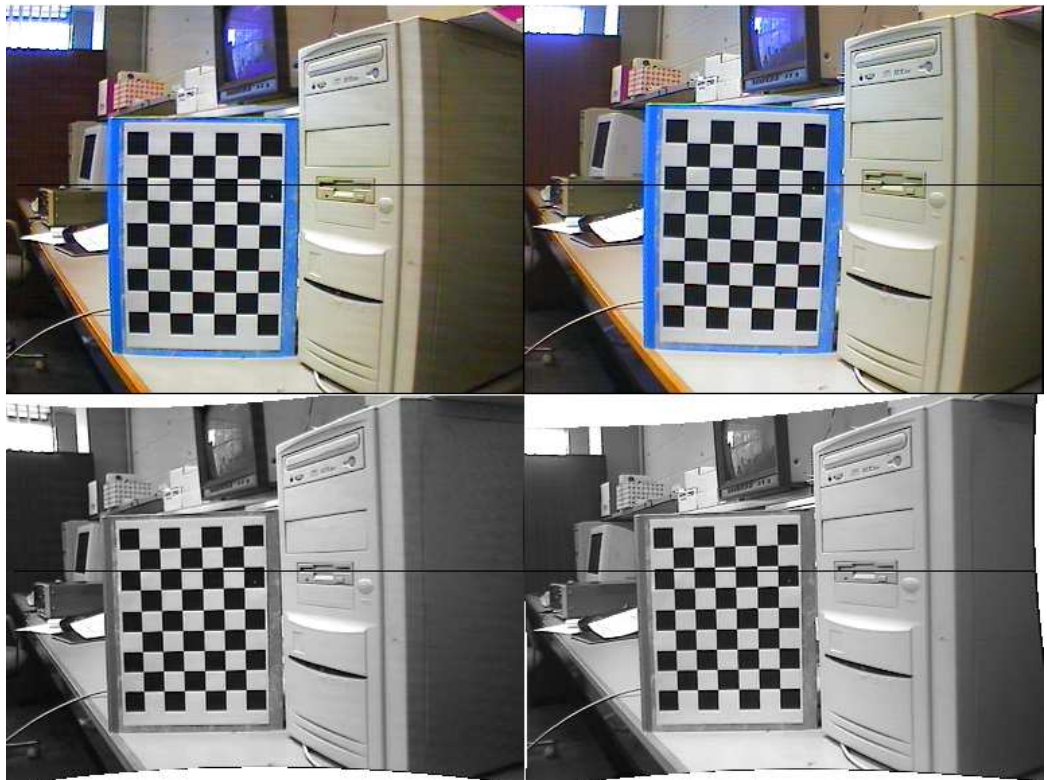
Figure B.5: Top: pair of images taken by our stereo rig. Bottom: the same pair after standardisation. Black lines have been drawn to exhibit the alignment of the corresponding image elements.
