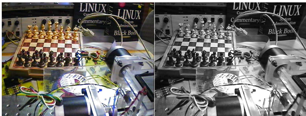
Figure B.4: The right image is the rectified left image. Notice that the power supply edge highlighted in previous figure appears straight.
