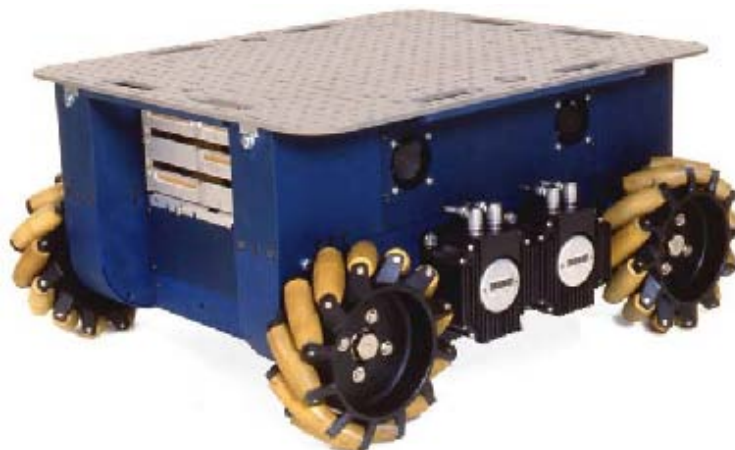
Figure 2.10: Uranus, CMU: Omnidirectional Drive with 4 Wheels.
