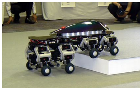
Figure 2.16: Halluc is a wheeled walking robot developed at Chiba Institute of Technology [22].
