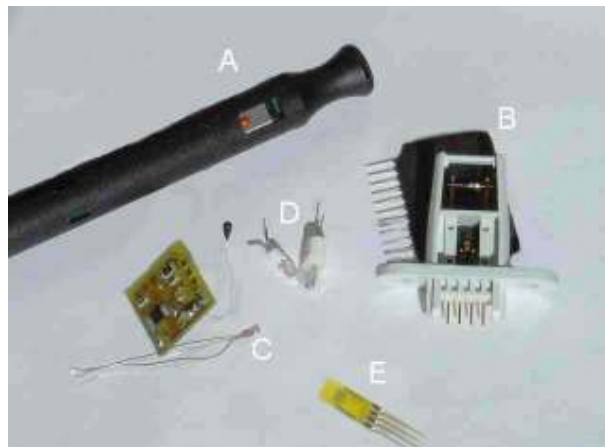
Figure 4.7: Some examples of sensors used to measure airflow - (A) Sensor from a Testo 435 anemometer; (B) Hybrid integrated circuit and sensor from Shibaura F6201-1 anemometer; (C) Commercial thermistors and signal condition circuit; (D) Tungsten wiring from a low voltage incandescent light bulb; (E) Thin film sensor from E+E Elektronik. [50]
