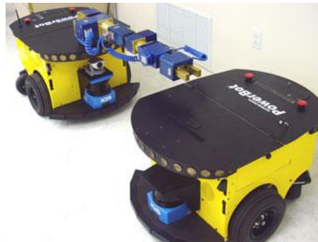
Figure 2.24: POWERBOT is a high-payload high-speed highly maneuverable platform [30].
