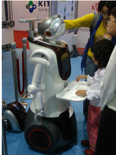
Figure 2.3: A semi humanoid robot which moves on 2 wheels with the differential drive concept.
