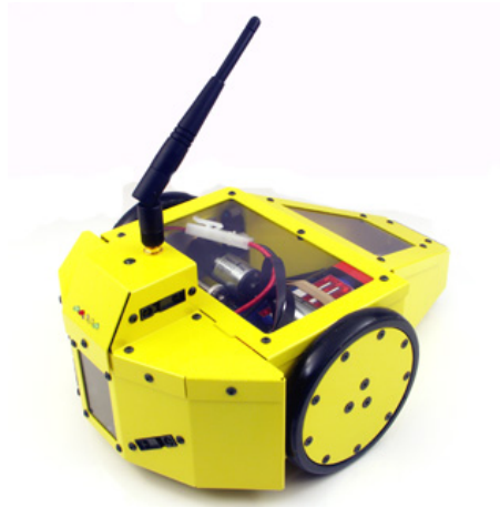
Figure 2.2: Garcia is canonical differential drive platform [6].
