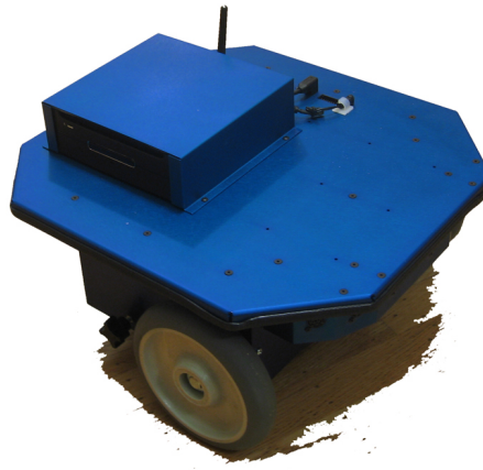
Figure 2.21: Erratic is a new mobile platform developed by Videre Design Co. [31].
