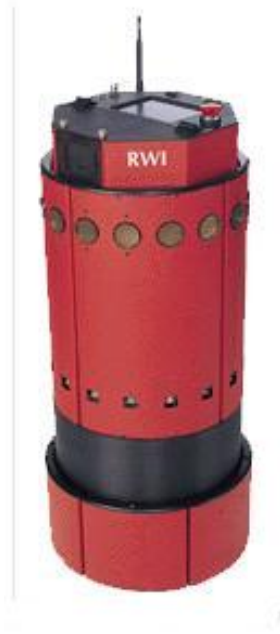
Figure 2.8: B14 is a synchrodrive mobile platform from RWI.
