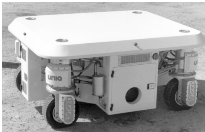
Figure 2.12: An 8-DOF platform with four wheels individually driven and steered. This platform was designed and built by Unique Mobility Inc. [5]
