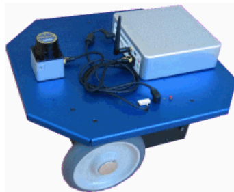
(a) Mobile platform Erratic: H8S controller, Servo and analog/digital I/O, 3x 7A 12V batteries. Onboard PC: 1.4 GHz Celeron, 802.11b/g, USB 2.0, IEEE 1394b, 40 GB, 512 MB
