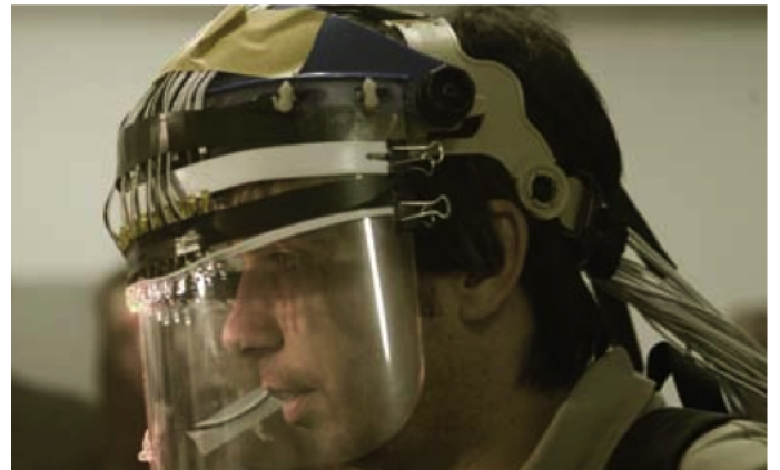
Fig. 6. Firefighter's Helmet that gets the goals from the base station and show them to the firefighter using color patterns
