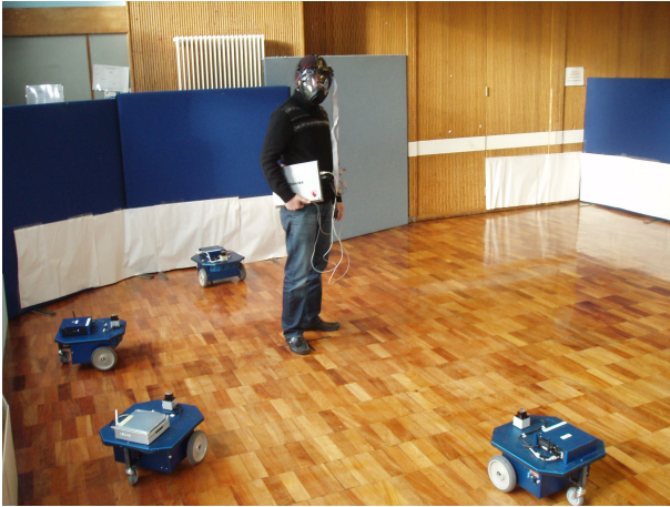
Fig. 2. Team of robots that maintain a flexible formation around the firefighter
