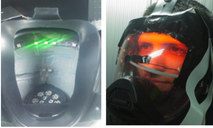
Fig. 11. Light Array Visor [LAV2] using real fire fighting helmet
