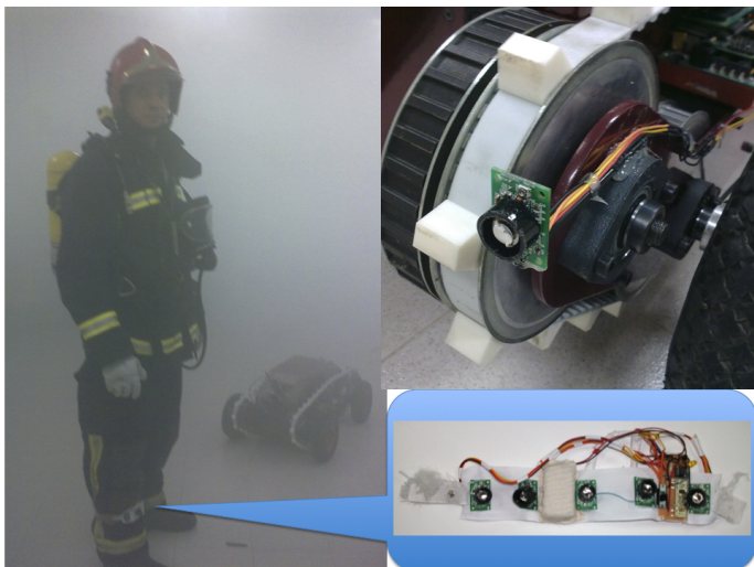
Fig. 4. Radio/Sonar firefighter localization and following in smoke using radio/sonar TDoA.
