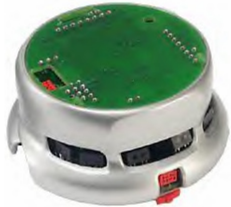
Figure 2: Khepera II Robot; is a 70 x 30 mm, 80g Robot with 8 IR sensors and 512 KB RAM.
