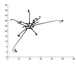
Fig. 2. Trajectories of the agents of a 10-agent swarm during the aggregation process.
