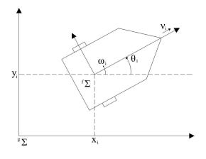
Fig. 1. The unicycle robot.
