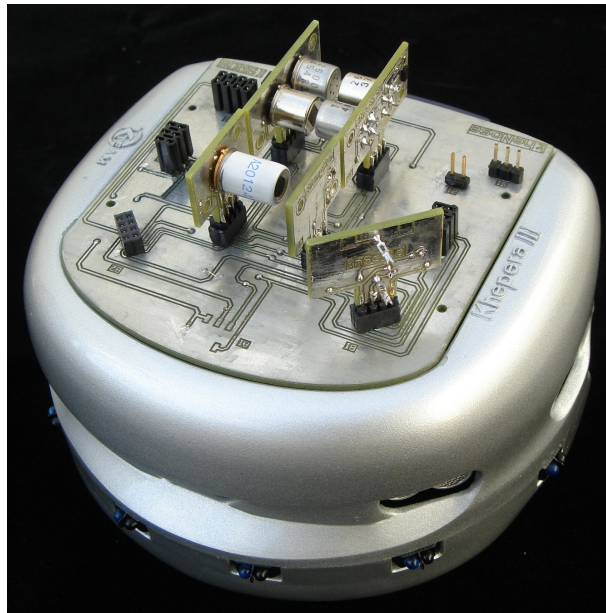
Figure 4.1: Khepera III and kheNose with sensing modules
