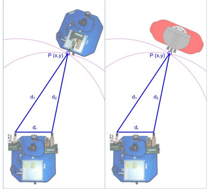
Fig. 12. Position determination by trilateration
