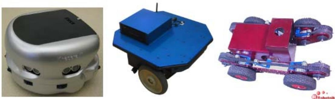
Figure 1 Robots in the Guardians project: Khepera III, Erratic and Robot Guardian.
