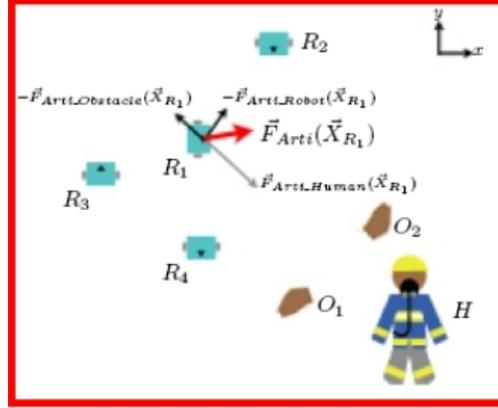
Figure 7 Forces acting on a robot.
