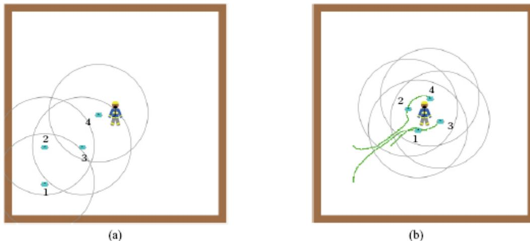
Figure 16. A chain of robots with limited visibility domains.
