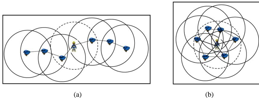
**Fig. 3.** Two examples of human-multi-robot formations: (a) Maximal formation, (b) Minimal formation. The visibility domains of robots are indicated as circles with solid boundaries, and the (passive) visibility domain of the human is depicted as a circle with the ‘dashed’ boundary
