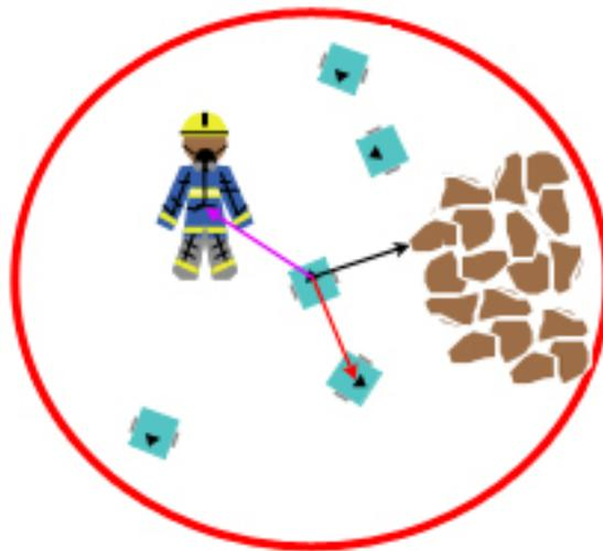
Figure 3 Visibility domain of a robot.
