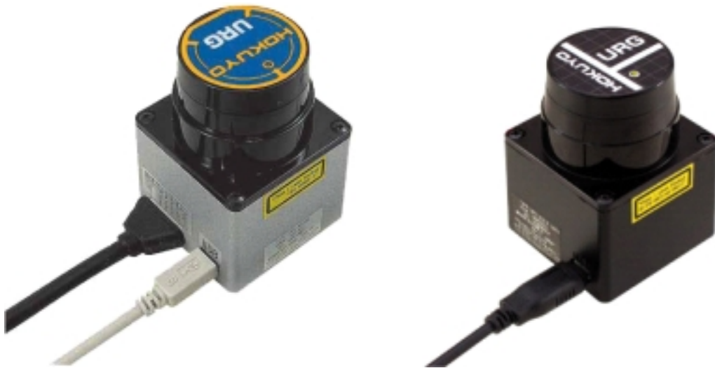
Figure 24: Two models of Hokuyo LRF. Left: URG-04LX, Right: URG-04LX-UG0
