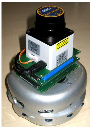
Figure 26: Khepera III and Hokuyo's LRF.
