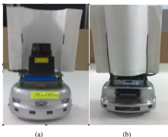
Figure 27: Khepera III robots with extra shape for laser detection (a) Front view. (b) Rear view.
