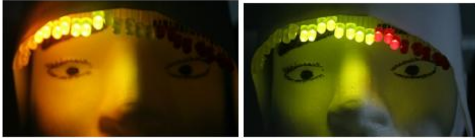
Figure 4: Early prototyping of LED activation system, depending on the message to pass to the fireman (by SHU)
