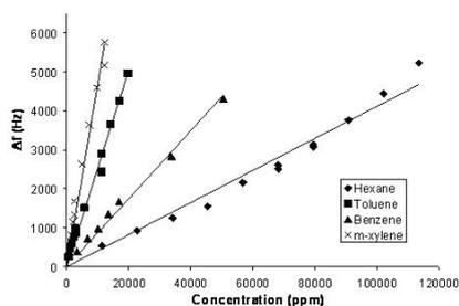
**Fig. 3.** QCM response to a range of VOC's.
