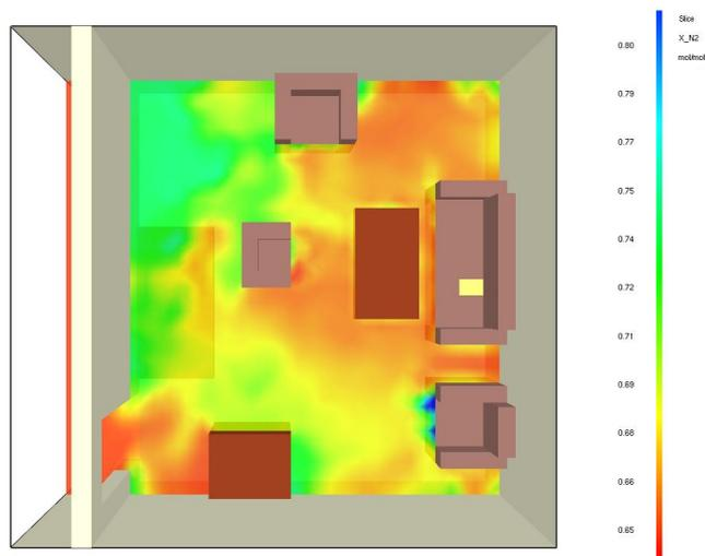
**Fig. 1.** Example 2D plot of a room with chemical sensor data superimposed. The colour-bar denotes the volume fraction of  $N_2$  in the mixture fraction of other chemical components
