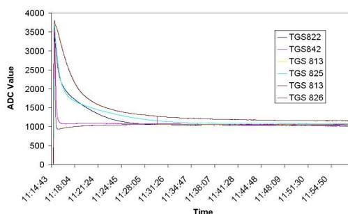
**Fig. 4.** Startup / initial action of several MOS sensors
