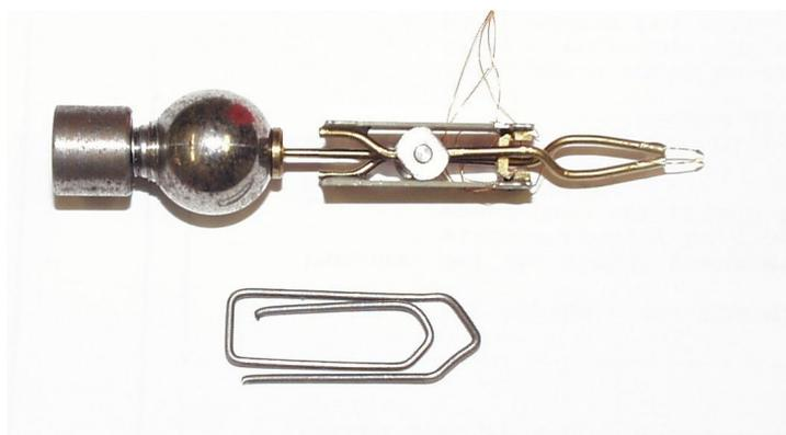
Figure 14: Two-fingered gripper, driven by bimorphic piezoactuators
