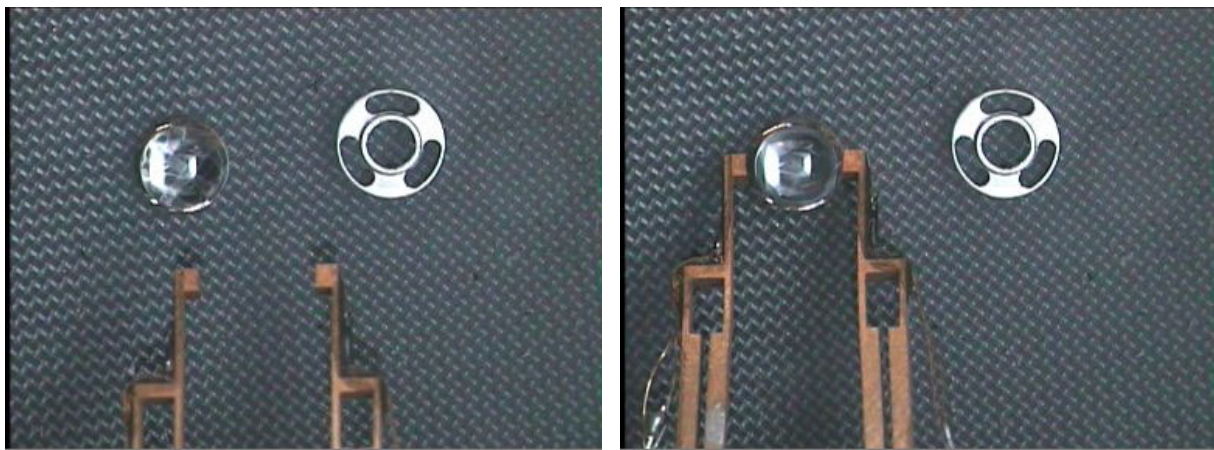
Figure 54: Picking up the main lens from the Gel-Pak
