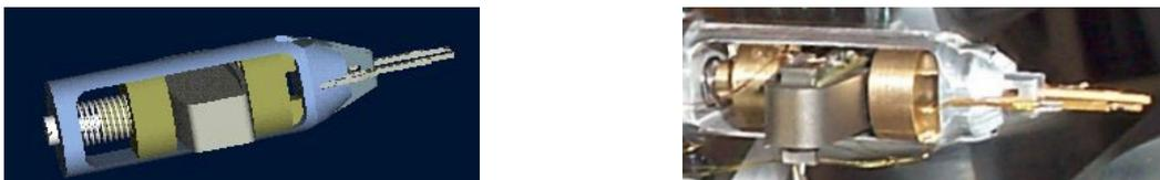
Figure 12: Gripper assembled in the symmetrical aluminum and brass mounting
