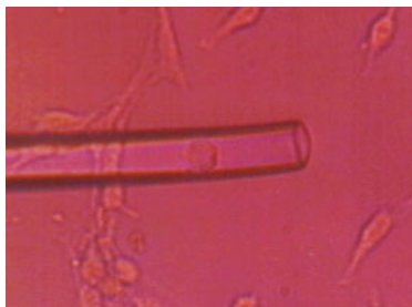
Figure 6: Cell handling with a 21 \mu\text{m} pipette
