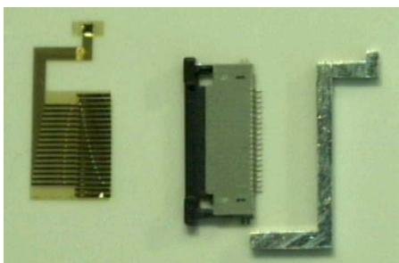
Figure 24: Complete tactile sensor with scheduled connector and finger of the Three Finger Gripper
