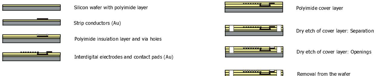
Figure 23: Improved process for the microfabrication of polyimide substrate
