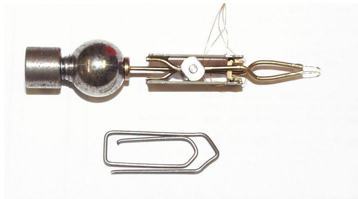
Figure 14: Two-fingered gripper, driven by bimorphic piezoactuators
