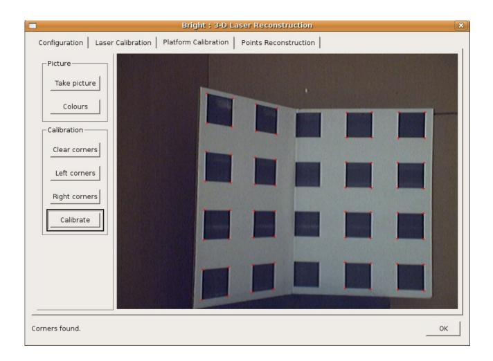
Then, take a picture with "*Take Picture*", and provide the values of black and white as usual with the button "*Colours*". Then click on the four extreme corners of the left chessboard, and click on "*Left corners*". Do the same with the right corners and the button "*Right corners*".
